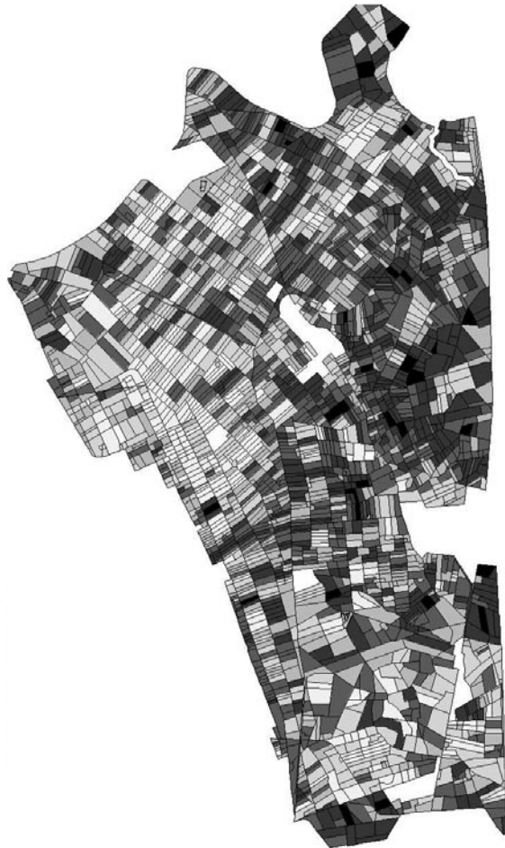
Figure 2. Vector map of potential evapotranspiration ETC of irrigated parcels derived from the LAI map of Figure 1 and ground-based meteorological data.
